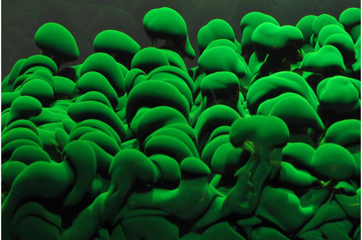
Figure 2.4: An example image of the Rayleigh Taylor instability. The green fluid is lower density fresh water and the clear fluid is higher density salt water. Image by Megan S. Davies Wykes from the University of Cambridge. The image may be found at http://www2.eng.cam.ac.uk/~msd38/gallery.html and the associated paper is Ref. [2].
