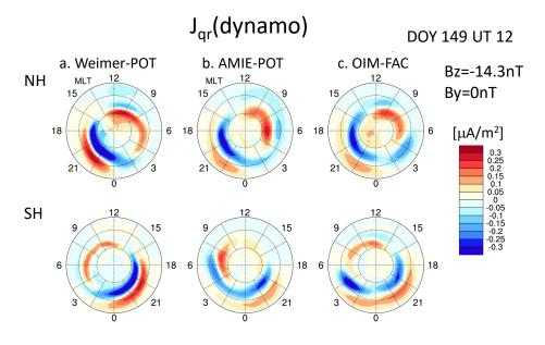
Figure 6. Radial current density  $J_{qr}$  [ $\mu A/m^2$ ] (positive is upward) for 29 May 2010 (day of year 149) at 12 UT due to the wind dynamo based on TIEGCM simulations for a. Weimer-POT, b. AMIE-POT, and c. OIM-FAC cases for the northern hemisphere (NH, top panels) and southern hemisphere (SH, bottom panels) over MLT and magnetic latitude (perimeter is  $\pm 50^{\circ}$  magnetic latitude).
