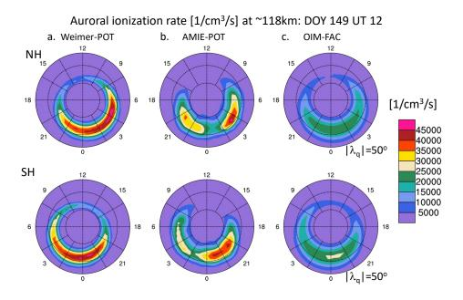
Figure 2. Auroral ionization rate  $\left[\frac{1}{cm^3s}\right]$  poleward of  $\pm 50^o$  quasi dipole latitude for 29 May 2010 (DOY 149 UT 12) for a. Weimer-POT case, b. AMIE auroral precipitation, and c. OIM-FAC case for northern hemisphere (top) and southern hemisphere (bottom) with Weimer-POT case and OIM-FAC case using the TIEGCM default analytical aurora model but with different parametrization (see Supporting Information)(Roble & Ridley, 1987).
