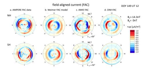
Figure 3. Field-aligned current  $[\mu A/m^2]$  (positive is upward) for 29 May 2010 (doy 149) at 12 UT plotted over magnetic local time (MLT) in northern hemisphere (NH, top panels) and southern hemisphere (SH, bottom panels) from different sources: a. AMPERE FAC data product [http://ampere.jhuapl.edu/], b. empirical Weimer FAC model (Weimer, 2005), c. FAC from AMIE procedure, and d. FAC using OI method. Note that these patterns are not based on TIEGCM simulations.
