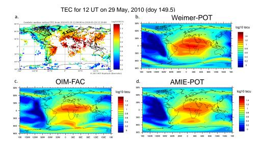
Figure 17. Comparison of total electron content (TEC) at doy 149.5 (29 May 2010 at 12 UT): a. GPS TEC from MIT Haystack observatory, b. Weimer-POT simulation, c. OIM-FAC simulation, d. AMIE-POT simulation.
