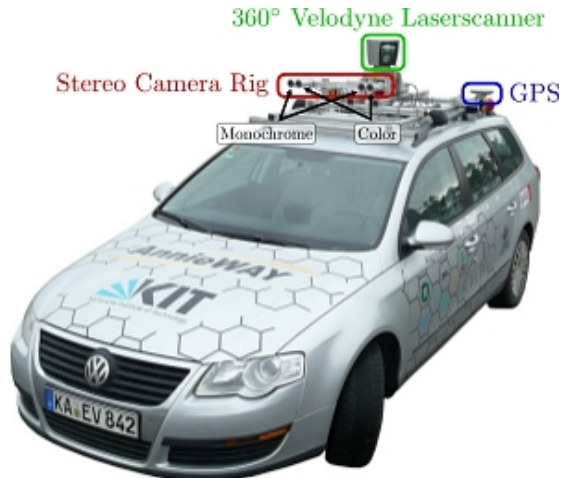
Figure 4.1: Volkswagen Passat B6, KITTI sensor setup. [7]
