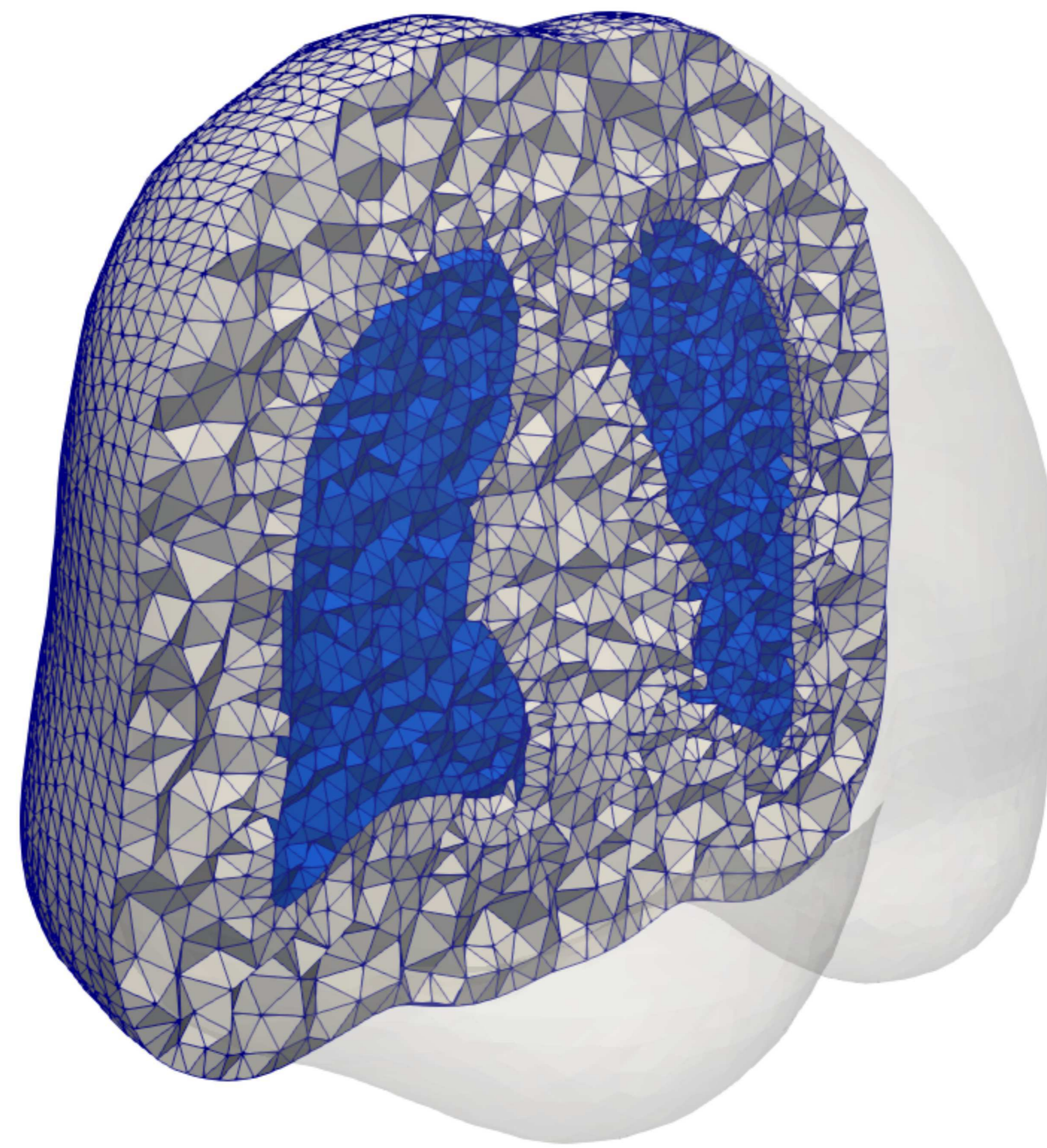
Linear elastic finite-element modeling Lungs + Body + Contact surface
