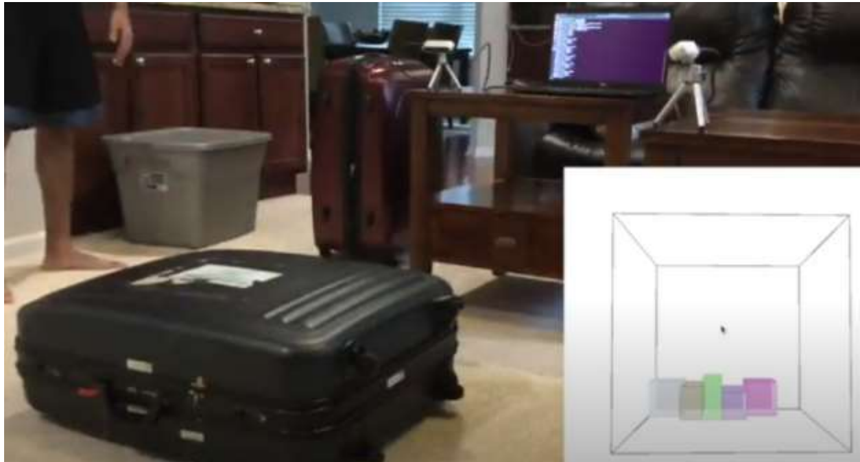
Figure 3: A view of our system running in a lab setting. Objects are placed in the staging area on the left, while the visualizer in the lower right shows placed items within the virtual container.
