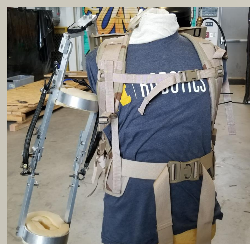
Figure 2. Current SAM-E design containing malleable cuffs with padding, as well as adjustability.
