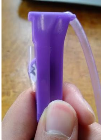
Figure 6. Potential solution — tape fixing roller clamp wheel to roller clamp IV housing.
