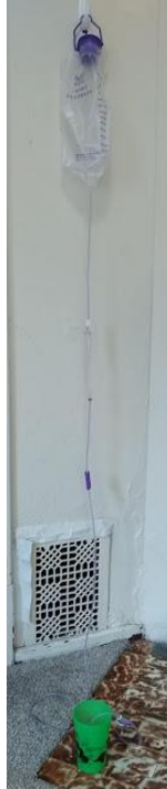
Figure 10. IV bag and tubing setup, with bag attached to wall hook and water draining into a cup on the floor.
