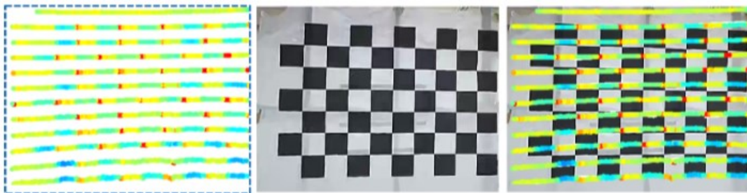
Figure 4.6: Corners of checkers on point cloud.
