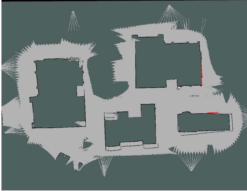
Figure 4.16: 2D grid map generated from Gamapping of simulation.
