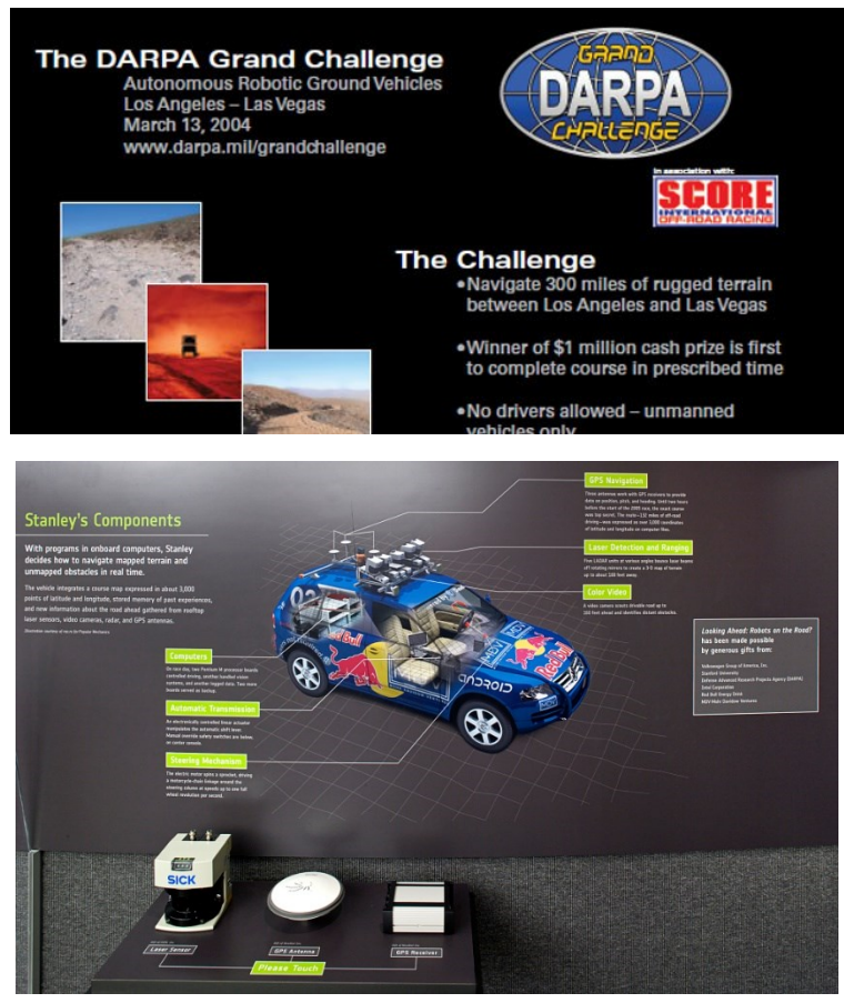
Figure 1.3: Poster for First DRAPA Grand Challenge (top side), and some of the hardware structure of Stanley, the entrant vehicle developed based on a Volkswagen Touareg. Image credit: The DARPA Grand Challenge: Ten Years Later via DRAPA.
