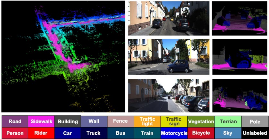
Figure 2.9: One typical application of data fusion, 3D object co-detection and segmentation. The segmented parts also have semantic information. [33]
