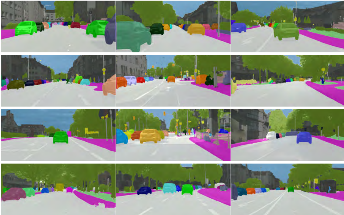
Figure 2.6: Panoptic segmentation results on Cityscapes val dataset. Results obtained with ResNet-50 encoder using a separate neck architecture, wBCE + Huber loss combination, split and merge refinement with min Instance area = 300 pixels. Instance contours ground truth are generated with dilation rate = 2.
