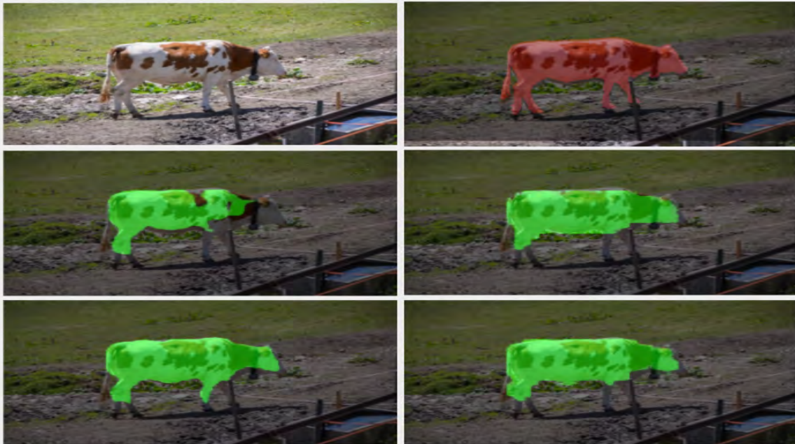
Figure 3.10: Results over DAVIS dataset. Left to right: RGB image, ground truth, single encoder (FCN), two stream encoder (MSFCN-2), two stream encoder + LSTM (RFCN-2), three stream encoder (MSFCN-3).
