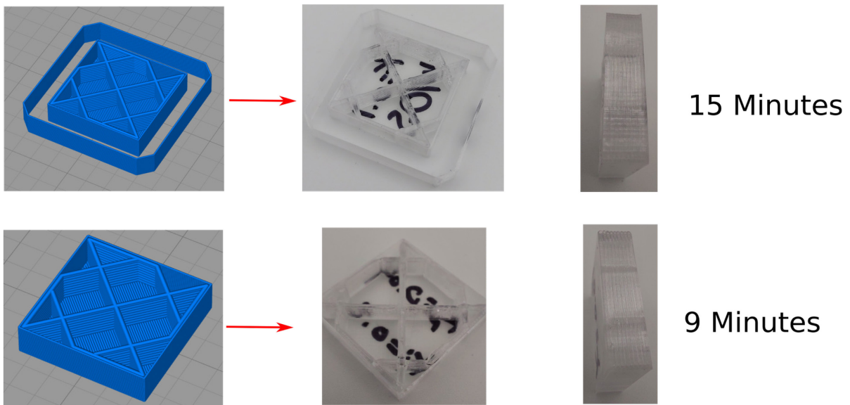
Figure 31 Half cube print results using an ooze shield.
