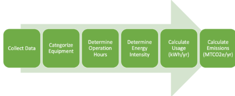
Figure 4: Flow chart depicting general process to calculate consumption and emissions of each system
