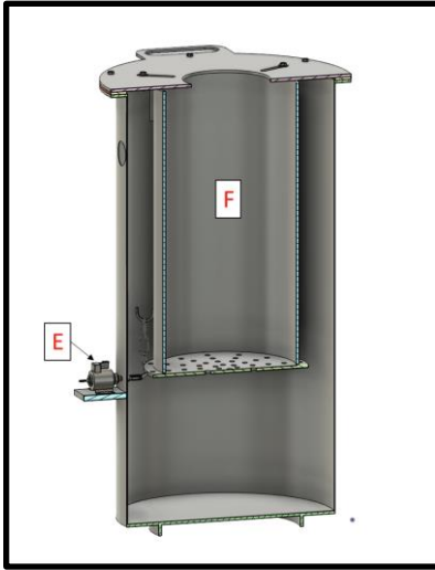
Figure 7 - Reaction Chamber. E) Solenoid. F) Fire tube.
