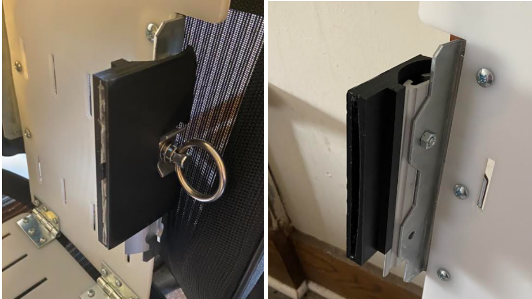
Figure 13: Outer and inner view of lateral support bracket with the O-track adjustability system attached to the frame of the device.
