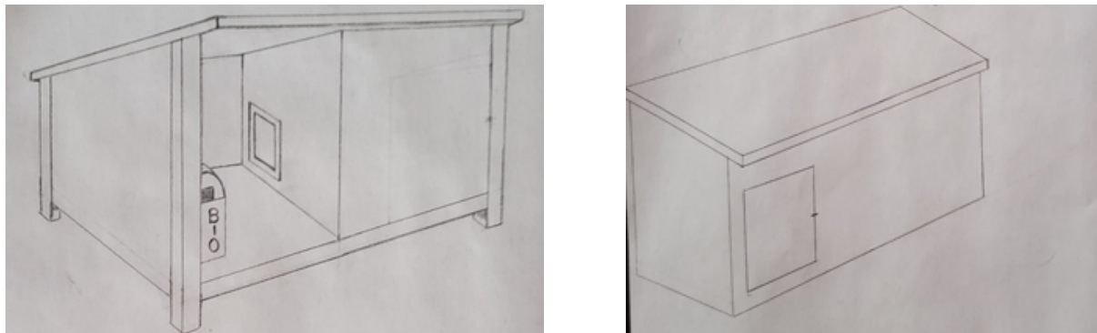
Figure 2: “Lean-to” design. Represented by Design 4 in the Pugh chart in Table 2. Pictured left is the front of the design showing the outdoor deck with access to interior via dog door. Pictured on the right is the back of the shelter which shows the back access hatch for cleaning.
