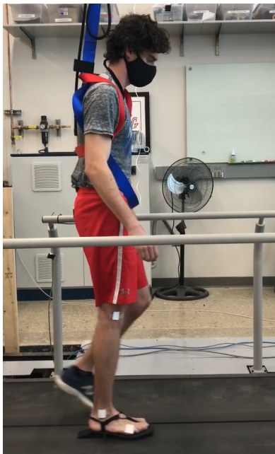
Figure 18. Team member, Aidan, walking on the treadmill with embedded force plates in the biomechanics lab. He is wearing the Springblade design with sandals supplied by the sponsor.
