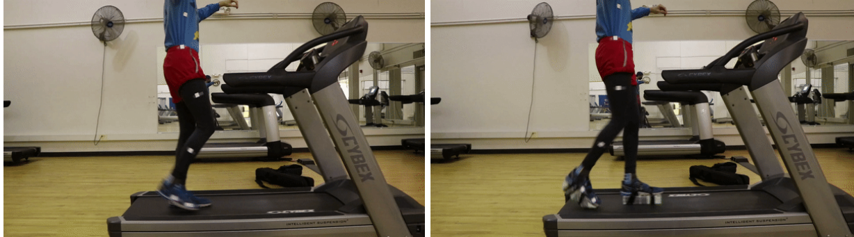
Figure 14. The tripod set-up to collect video footage of normal gait (left) and gait with the prototype Disco Shoe (right). The white squares are placed along the legs for tracking purposes during analyses.
