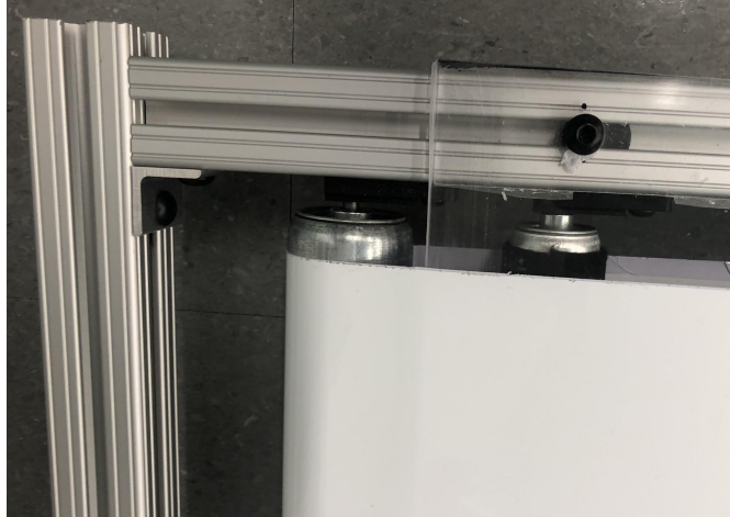
Figure 22. View from the top left of the system, a reminder of the respective location of the middle roller, which can be seen coated in a layer of black colored felt.
