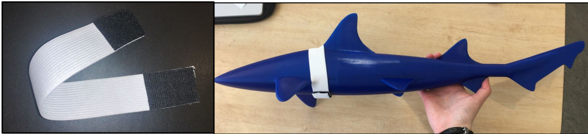
Figure A3.1: Images of the first Shark Belt proof of concept, consisting of one elastic band to be placed in front of the first dorsal fin.
