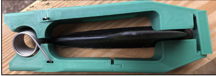
Figure A2.12: Top view of the clip attached to a model fin.
