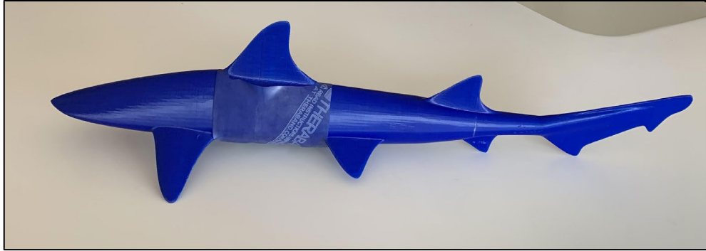
Figure 10: Image of shark “vest” surrounding the first dorsal fin. Vest is secured under the dogfish with Velcro®.
