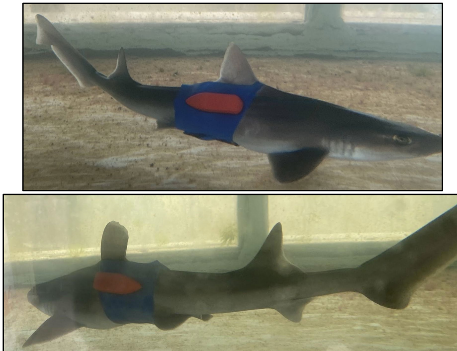
Figure 34: Final Prototype on the dogfish at WHOI. (Top) The whole tag slid back on the body and put stress on the front of the first dorsal fin. (Bottom) The tag also decoupled from the dogfish body, multiple causes are possible [22].
