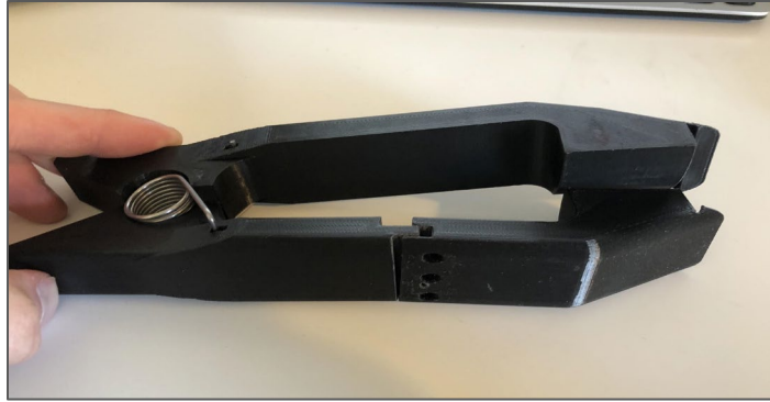
Figure A2.4: Side view of the 3-D printed model for Version 1 of the Fin Clip.
