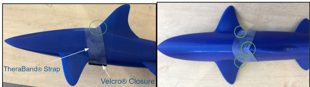
Figure 9: Single strap belt located forward of the first dorsal fin. (Left) Side view highlights interference with the dorsal fin and the Velcro® closure. (Right) Top view highlights interference with pectoral fins and dorsal fin.
