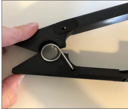
Figure A2.6: The clip with the spring installed, highlighting the incorrect placement of the center of rotation.
