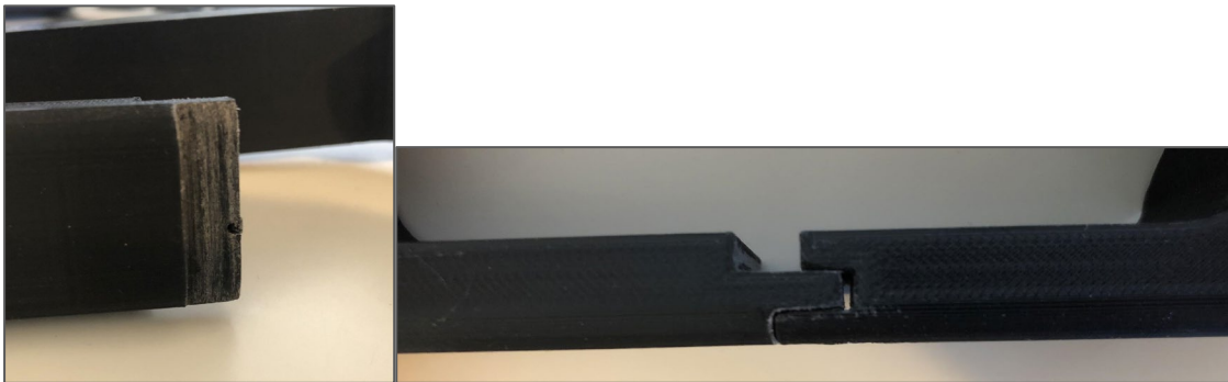
Figure A2.5: (Left) the Fin Clip tab surface that was sanded down. (Right) The parts fit together cleanly after sanding.
