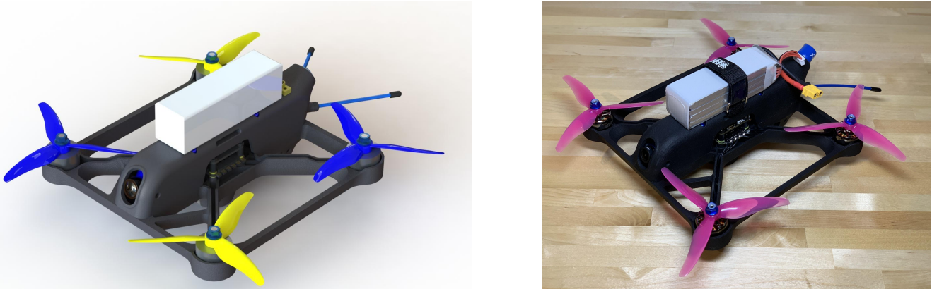
Figure 15. Side-by-side comparison of the drone in Solidworks versus assembled.
