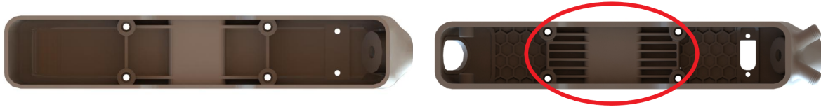
Figure 12. Initial (left) and final (right) top shell designs. Final top shell includes beam and hexagon reinforcement to lower the effect of impact force at the battery-shell interface.
