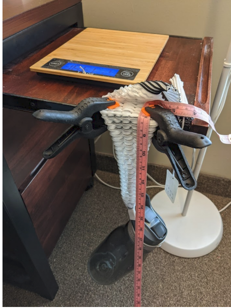
Figure 16. Experimental procedure to measure textile stiffness. A water bottle was used to apply various loads to the textile and a tape measure was used to measure the extension of the textile. The bottle was weighed using a kitchen scale.
