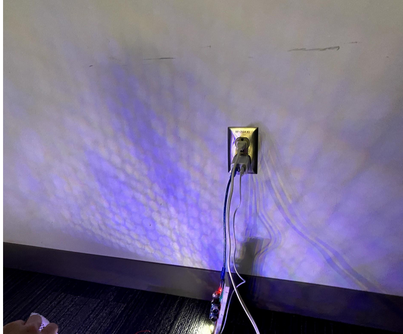
Figure 24. Mesh bag and 217lm LED lights. In this case, the lights were alternating purple and white. Due to the lower lumen rating, the projections were captured on a closer wall in order to gauge projection quality.
