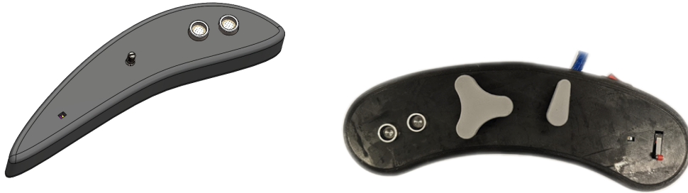
Figure 37. Initial design of control box (left) compared to final prototype (right). The final prototype is more rounded and larger than the initial design to accommodate additional components.
