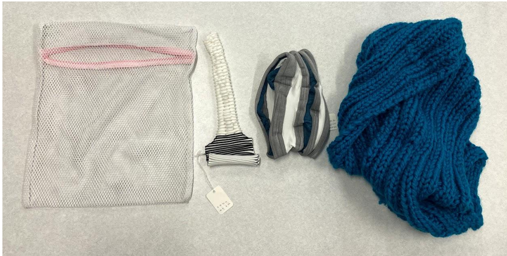
Figure 21. Textiles being tested from left to right: Mesh bag, nylastic and plastic filament textile, polyester knit, chunky knit scarf. The center two textiles were provided by Prof. Ahlquist's textile lab at Taubman.
