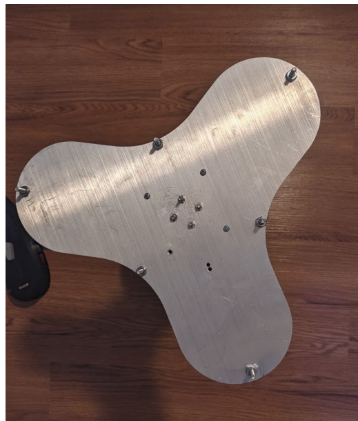
Figure 33. The shape of the top disk was modified to improve user engagement.
