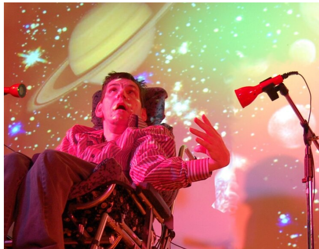
Figure 4. The Soundbeam. The red flashlight-shaped objects on the left and right of the figure are the “beams.” When the user crosses this beam with an object (i.e. an arm or hand), the device maps their motion to music. [4]
