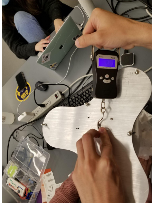
Figure 40. Torque test on top platform. A force was applied at a 1 inch moment arm. The handheld force gauge reads 4.3 lb.
