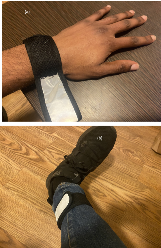
Figure 44: Wrist strap that comes with a built in mesh pocket to hold IMU.
