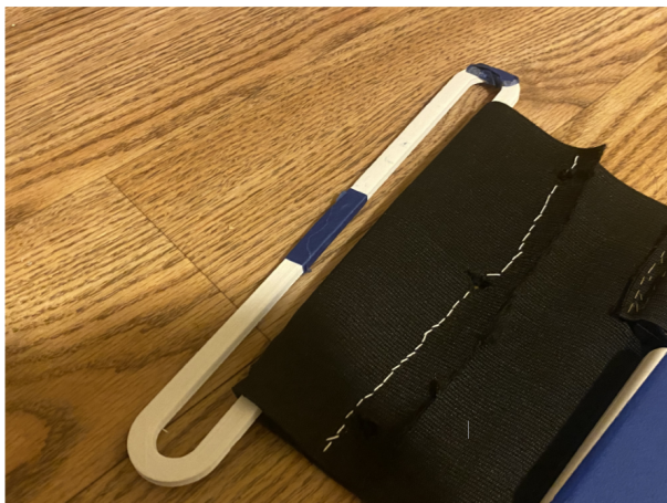
Figure 40: The 3D printed buckle for the torso strap.
