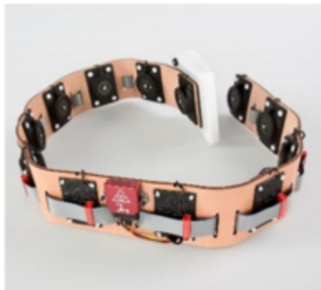
Figure A3.2 [17]: The device designed by Kingma et al. to be worn long-term as a belt to provide vibrotactile feedback on tilt angle.
