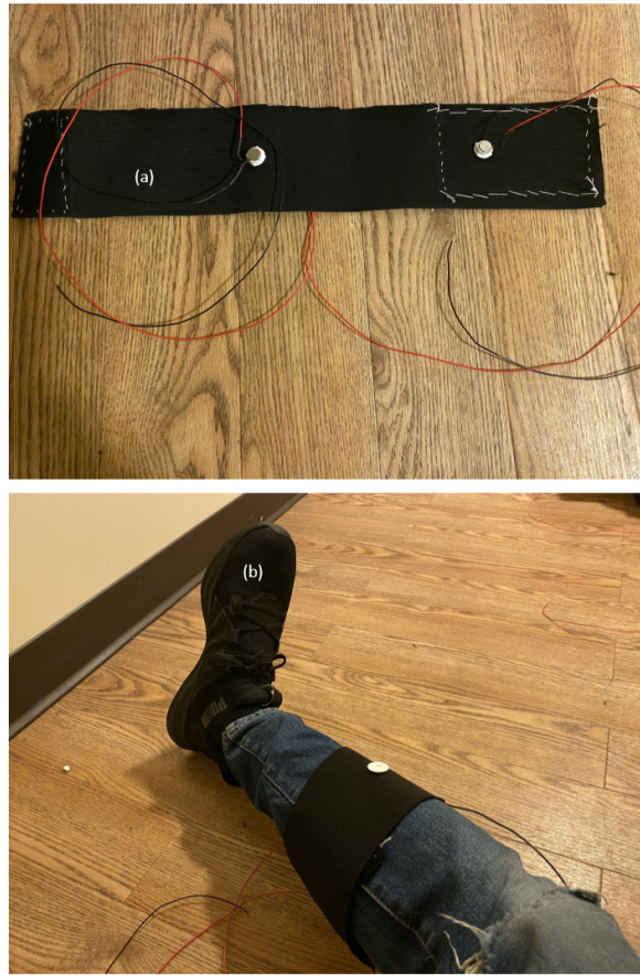
Figure 43: (top) strap design detailing posterior and anterior tactors for shin and calf biofeedback respectively. (bottom) strap component on device wearer with tactors interfacing with wearer's shin and calf.
