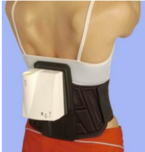
Figure A1.2 [23]: SwayStar™ is worn around the waist at the level of the lumbar spine and is held in position with a belt.
