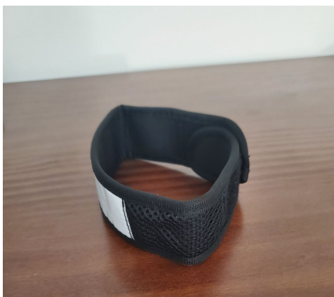
Figure 41: The ankle strap. It comes with a built in mesh pocket to hold the IMU.
