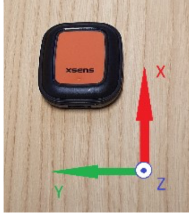
Figure 28: Xsens DOT local reference frame.
