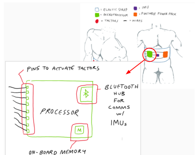
Figure 16: Additional sketch of the processor component. The processor will be located on the wearer’s lower back by attaching to the same elastic band that holds the tactors and portable power pack.
