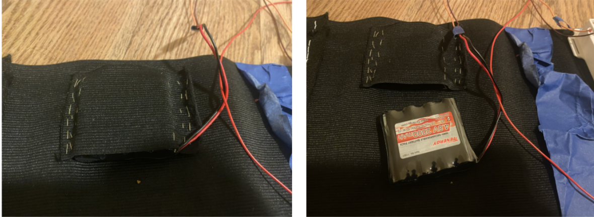
Figure 38: The pocket on the torso strap that holds the tactor power supply.
