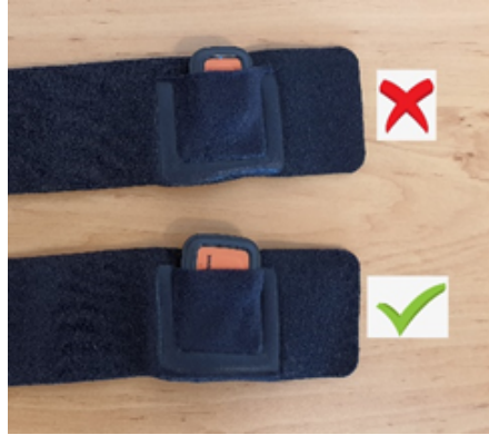
Figure 23: The IMU should be placed horizontally instead of vertical in the pocket of the strap to ensure a snug fit.
