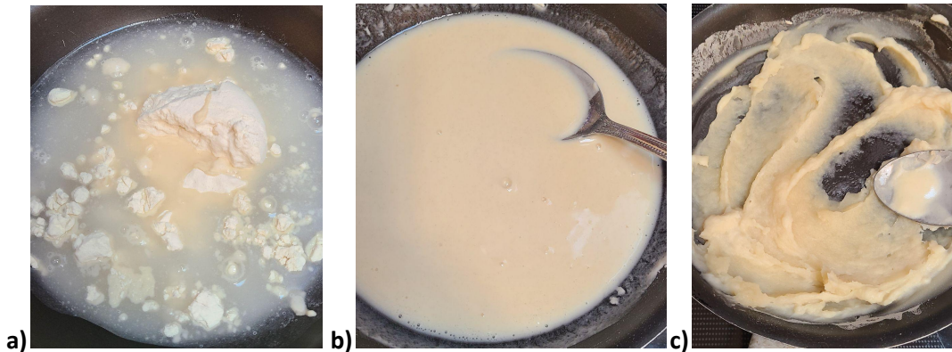
Figure E.1: Flour and water mixture a) initially b) after mixing and breaking up all clumps c) after being heated for 5-7 minutes
