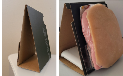
Figura E.12: a) Stand once it has been cut, folded and assembled. b) Fully assembled intramuscular injection simulator
