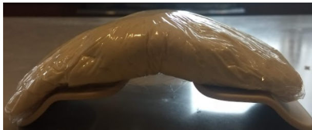
Figure 20. The first muscle and fat dough prototype, wrapped in plastic and propped to show potential shape and flexibility.
