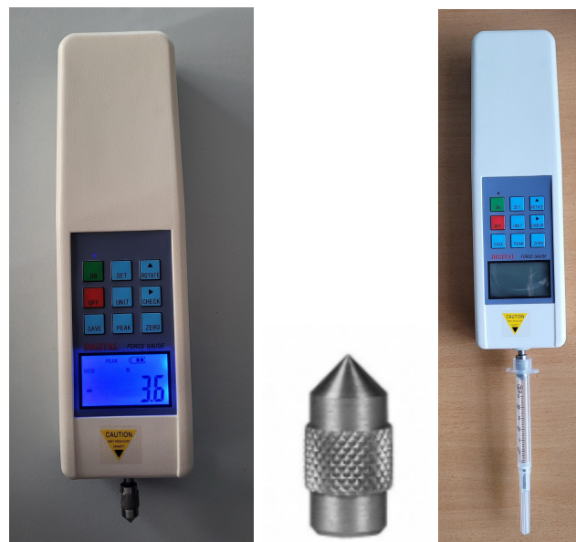
Figure 21. The HF-200 series Force Gauge with the attachment (left) that was used to record the force data for each of the layers. The attachment used to perform the tests (center). The attachment and syringe combination used to perform the second tests (right).
