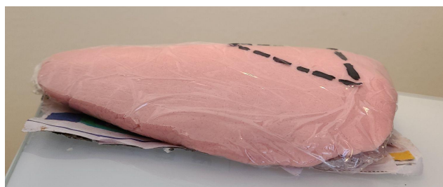
Figure 17. Muscle and fat dough prototype, wrapped in plastic with ideal injection location marked by the dashed triangle
