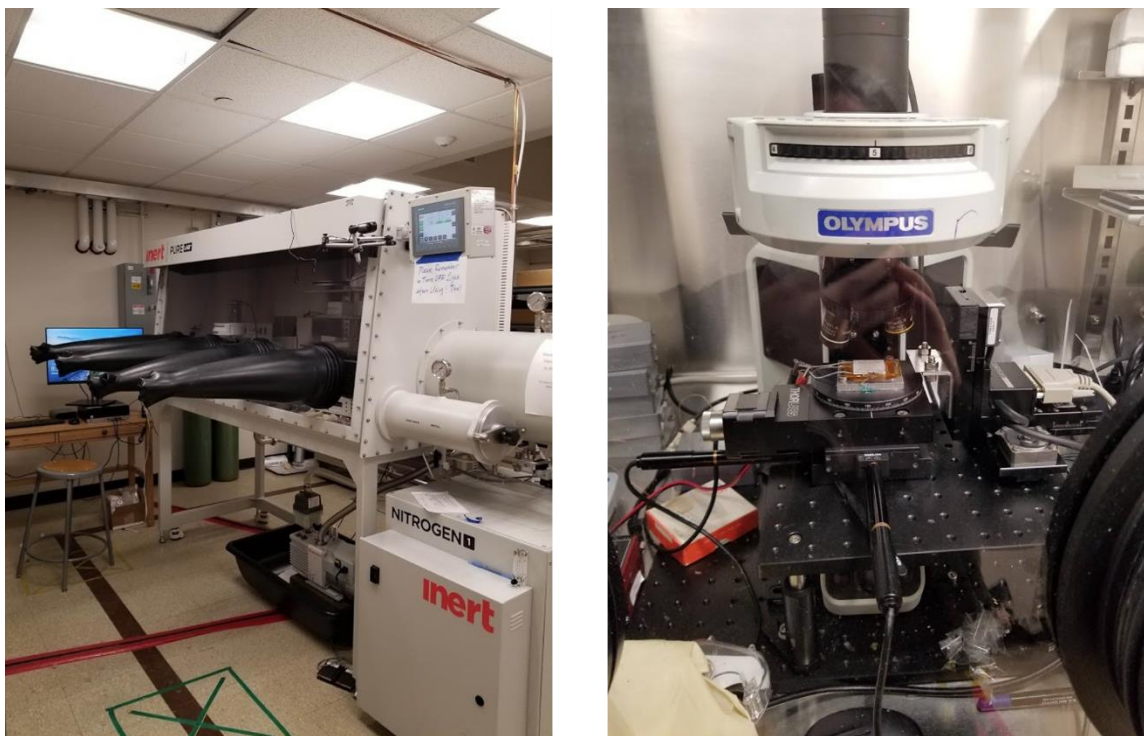
Figure IV.12 – Pictures of the glovebox-based 2d fabrication setup in the lab in the sub-basement of Randall Laboratory. (Left) The 4-glove Purelab HE from Inert. (Right) The Olympus microscope setup for the stacking procedure inside the glovebox. Two motorized stages from Thorlabs are shown to allow lateral movement of the sample within the focal plane. Atop these lateral stages is a Thorlabs rotation stage, on which is an aluminum sample mount with a thermal heating pad. Also pictured is the three-axis stage used to hold the microscope slide with the top stack for the stacking procedure.
