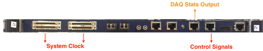
Figure 3.6: The MACTRIS+ front panel. The system clock is distributed to the L1 and L2 slave MACTRIS+ boards via the ribbon cable ports. The DAQ statistics are output to the L3 trigger via one Ethernet port and another Ethernet port distributes the control signals to the master fanout board.
