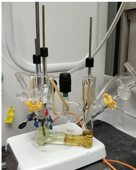
Figure A.92 The H-cell is used for controlled-potential electrolysis experiments in this study. The left chamber is filled with 20 mL MeCN solution of 0.3 mM [Co(PDI-R)] catalyst with 0.1 M n\text{Bu}_4\text{NPF}_6 , and the reported concentrations of \text{H}_2\text{O} . The glassy carbon plate working electrode and \text{Ag}/\text{AgNO}_3 (1.0 mM in MeCN with 0.1 M n\text{Bu}_4\text{NPF}_6 ) reference electrode are inserted into the solution. The right chamber is filled with 15 mL MeCN solution of 5 mM Fc with 0.1 M n\text{Bu}_4\text{NPF}_6 , and the same concentrations of \text{H}_2\text{O} as the left chamber. Nichrome wire is used as a counter electrode. Two chamber solutions are isolated by a fine-porosity glass frit.
