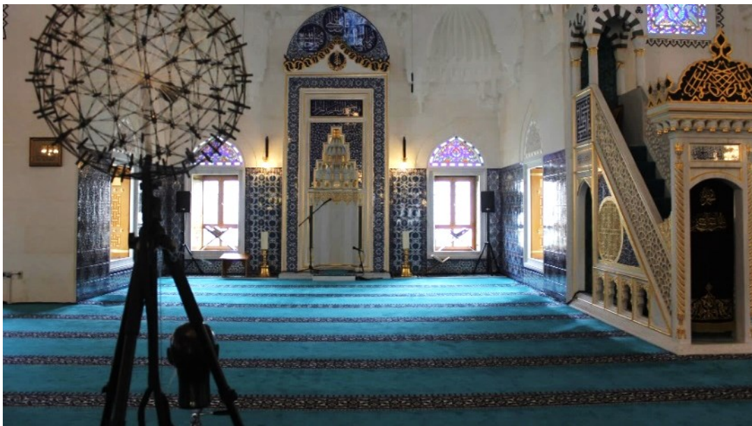
Fig. 3.4 Interior view showing the architectural features and the field measurement method (acoustic camera) at the Diyanet Center of America in Lanham, Maryland.
