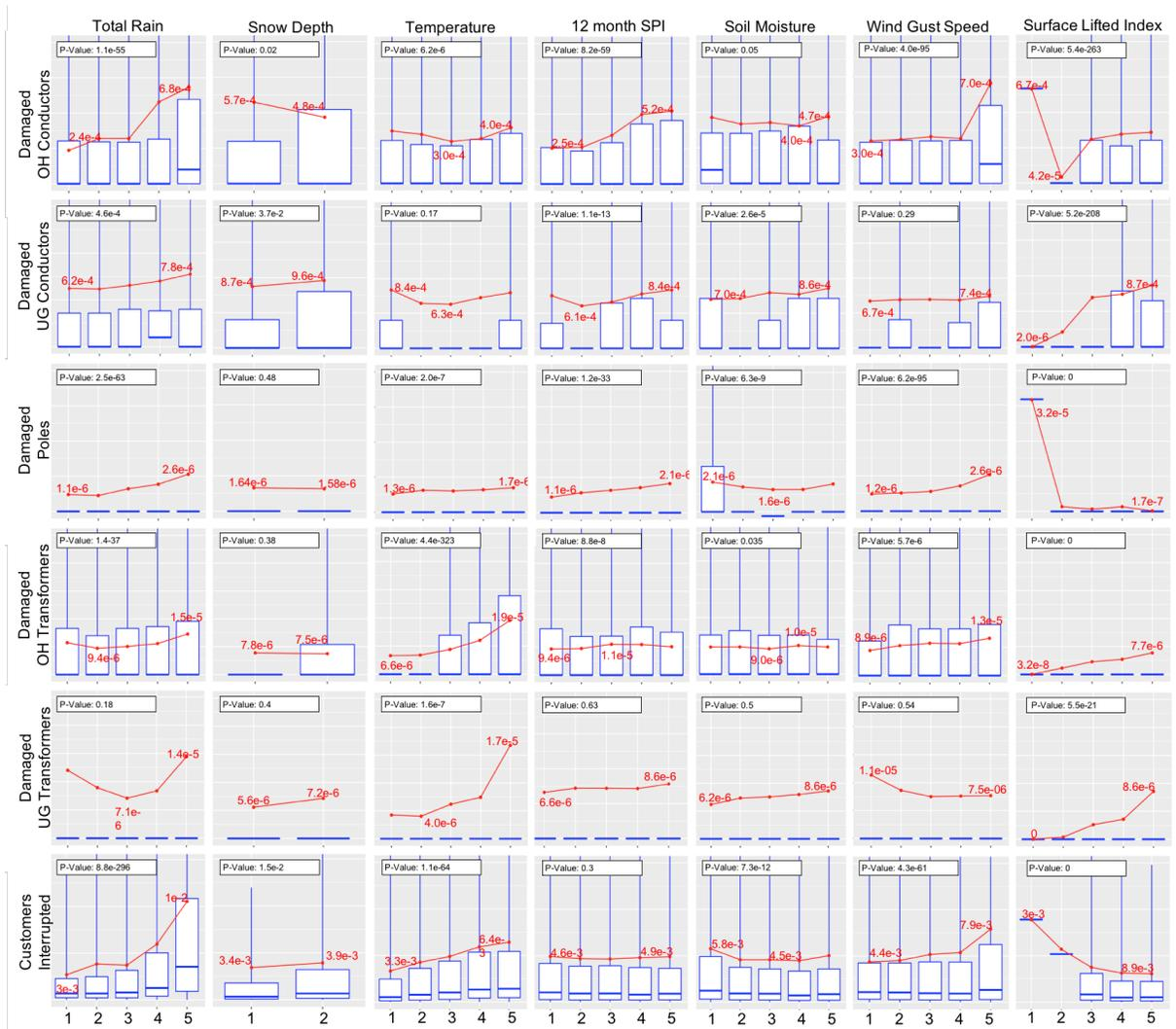
Figure 4.3: Results of the ANOVA test for each variable and damage type. The boxplots show the distribution of damages in various levels of each variable. The connected red points indicate the mean damage in each group. P-value of the ANOVA test, the maximum and minimum damage means are also shown in each sub-figure.
