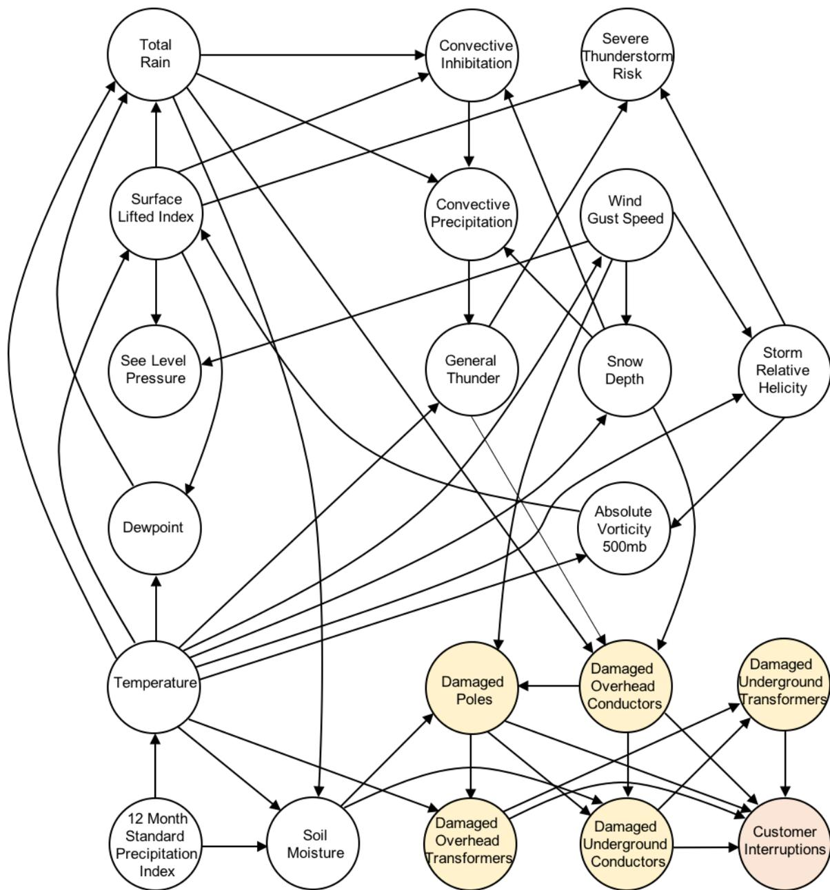
Figure 4.2: The Bayesian belief network representing the associations among meteorological variables (shown by white circles), damaged assets (shown by yellow circles) and customer interruptions (shown by brown circle) in the power grid.
