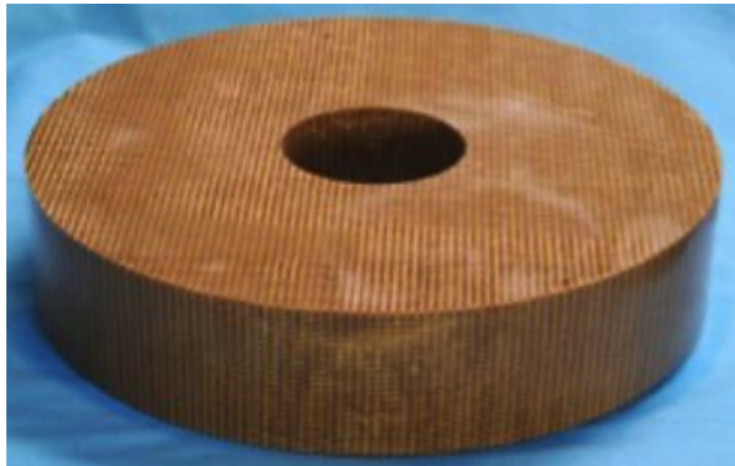
Figure 1.10: Flight compression pad made from 3D-MAT [3].
