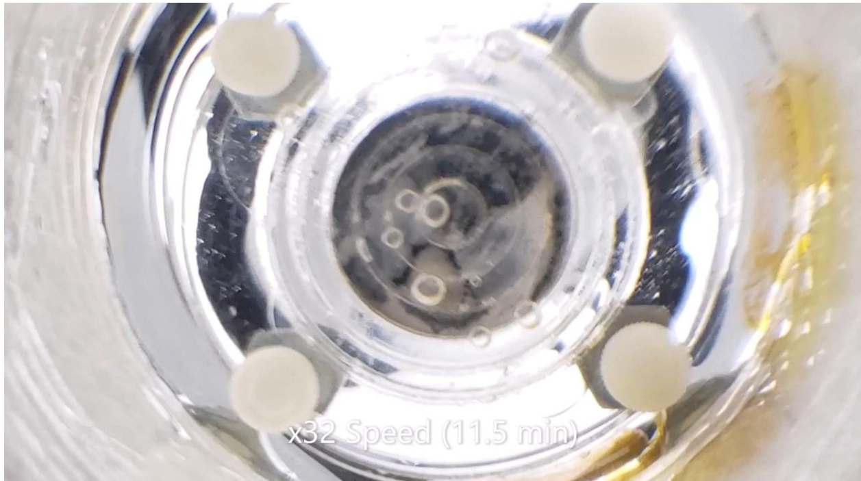
Figure 5.6: Lithium foil disk is placed in between two circular sheets of acrylic and exposed to water in an insulated vessel (Chamber #2), 11.5 minutes duration and x32 time speed.
