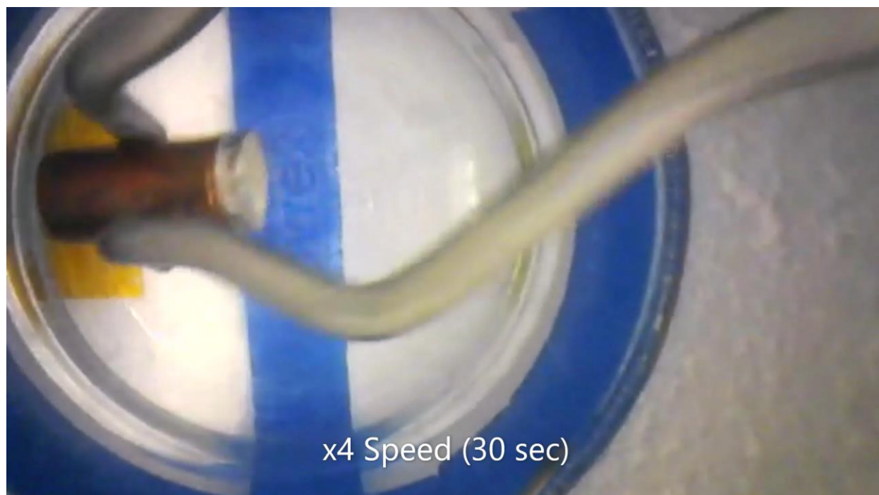
Figure 5.4: Lithium foil is attached to a copper weight to enable it to be submerged in water in an insulated vessel (Chamber #1), 30 second duration and x4 time speed.
