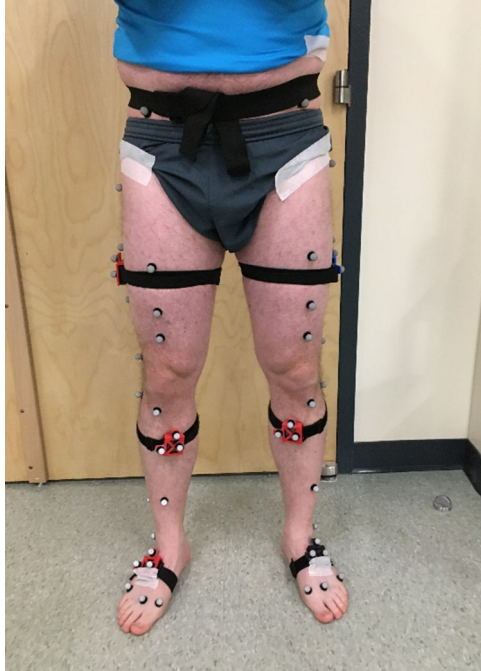
Figure 3.2: IMU and reflective marker placement for the stiff-legged walking experiment.
