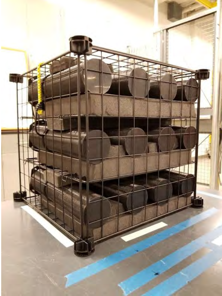
Figure 3.6: Photo of the OSCAR system, a 3 \times 4 array of stilbene detectors; figure from Ref. [3].
