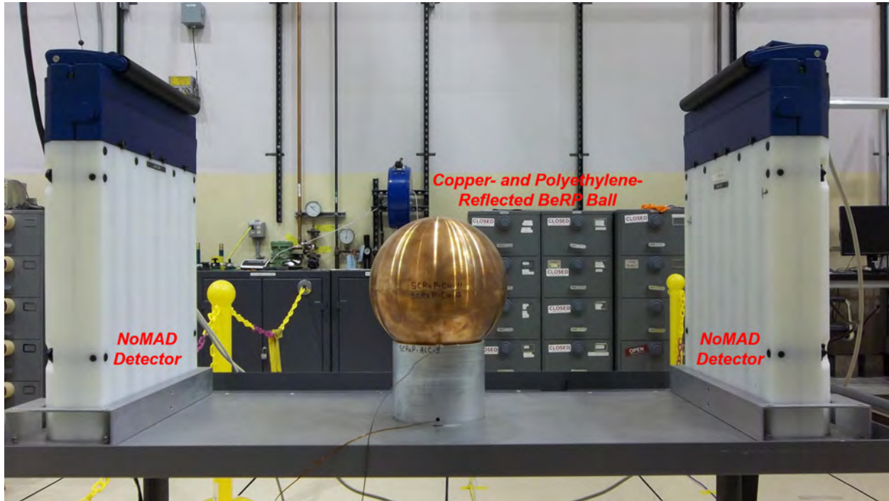
Figure 5.6: Photo of the experimental setup for the ^3\text{He} measurements.
