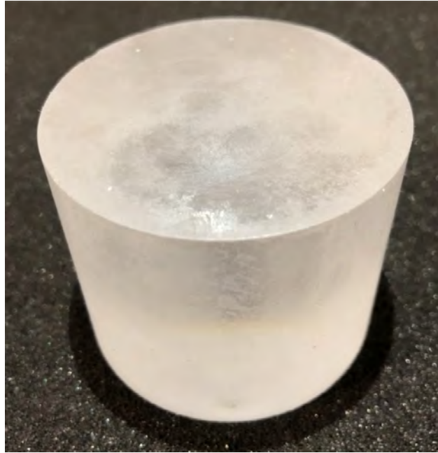
Figure 3.3: Photograph of a stilbene organic scintillator; figure from Ref. [2].
