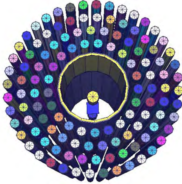
Figure B.2: Three-dimensional partial rendering of the ENMC; the moderating polyethylene is not shown.
