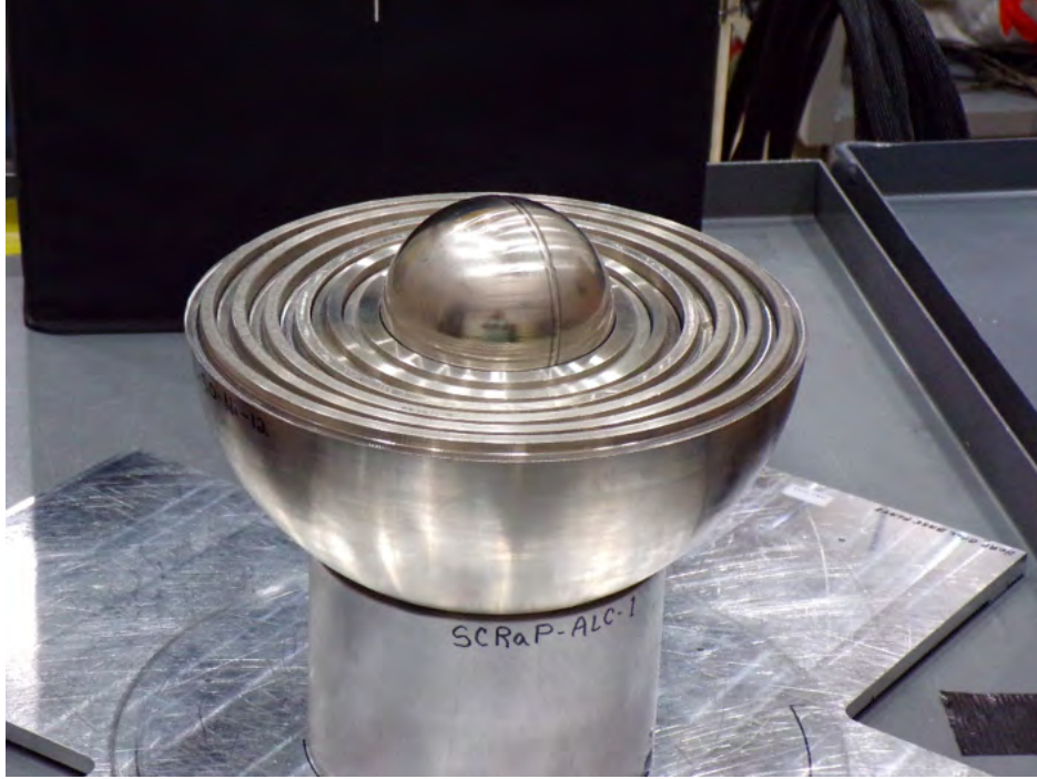
Figure C.1: Photograph of the 6-kg ^{237}\text{Np} sphere nested in the bottom half of the nickel hemishells.
