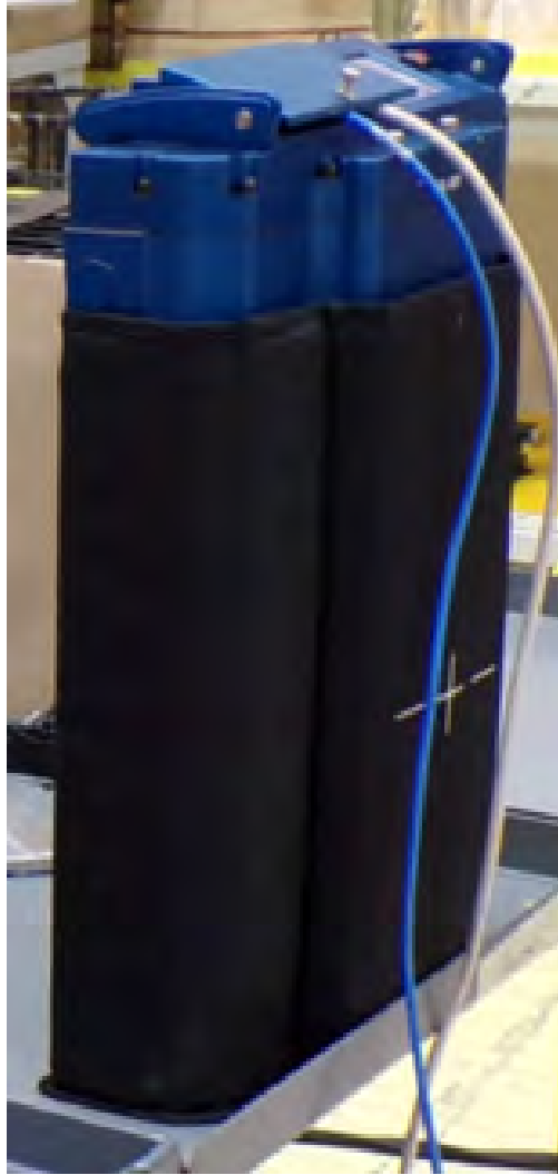
Figure C.2: Photograph of the Neutron Multiplicity ^3\text{He} Array Detector (NoMAD).
