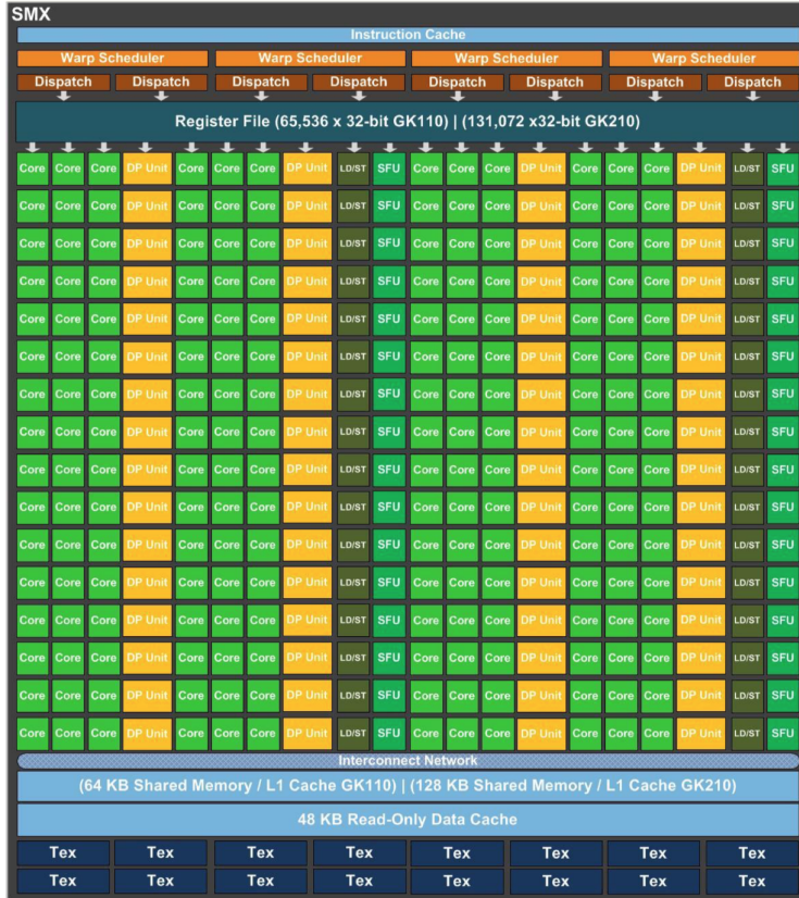
Figure 3.2: Structure of an SM on the Kepler GK110. The SM contains 192 cores which each have access to SM-wide shared memory, L1 cache, and read-only memory. Source: NVIDIA Kepler GK110/120 Whitepaper [76].
