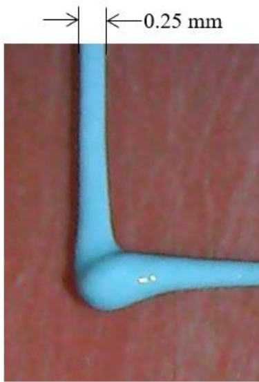
Figure 1.1:(a) Excess material deposition at a 90-degree corner produced by DIW where the material deposition was not matched with machine dynamics and (b) bulging corners on a DIW part.
