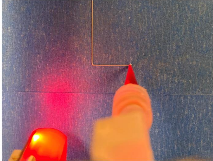
Figure 3.6: A 90-degree corner produced by the DIW system
