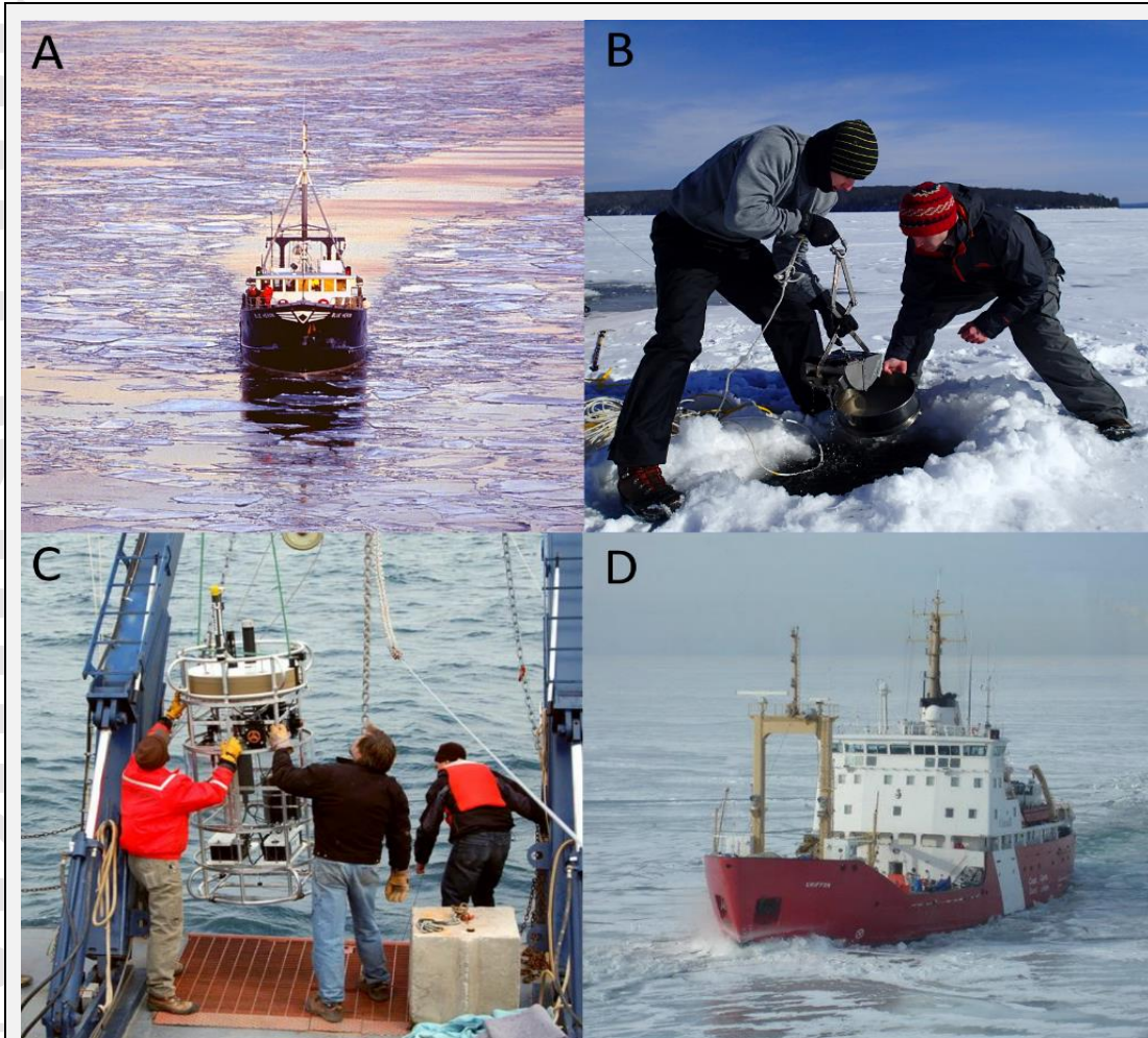
Figure 9: Several existing approaches to winter sampling in the Great Lakes. A) The University of Minnesota's R/V Blue Heron travelling through early spring ice on Lake Superior (photo by University of Minnesota Duluth); B) Researchers sampling benthos in the Apostle Island area of Lake Superior (photo by Ted Ozersky); C) A WetLabs AMP100 autonomous profiler being deployed in Lake Superior. The instrument travels up and down its mooring tether, recording water column parameters including temperature, oxygen concentrations and chlorophyll fluorescence (photo by Jay Austin); D) The Canadian Coast Guard icebreaker Griffon, which has supported winter limnology research on Lake Erie (photo by Paul Miller from Canada Steamship Lines).
