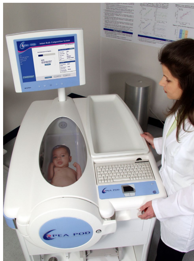
FIGURE 5 Pea Pod™ body composition system for infants. Photos used with permission from COSMED USA, Inc
