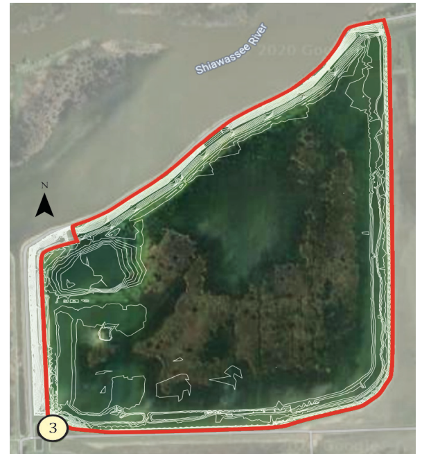
Figure 1.6: Aerial photo of MN. Gray lines represent water level topography. Point #3 indicates the water control structure that connects MN to the Shiawassee River. Image from Lugten et al. (2020).
