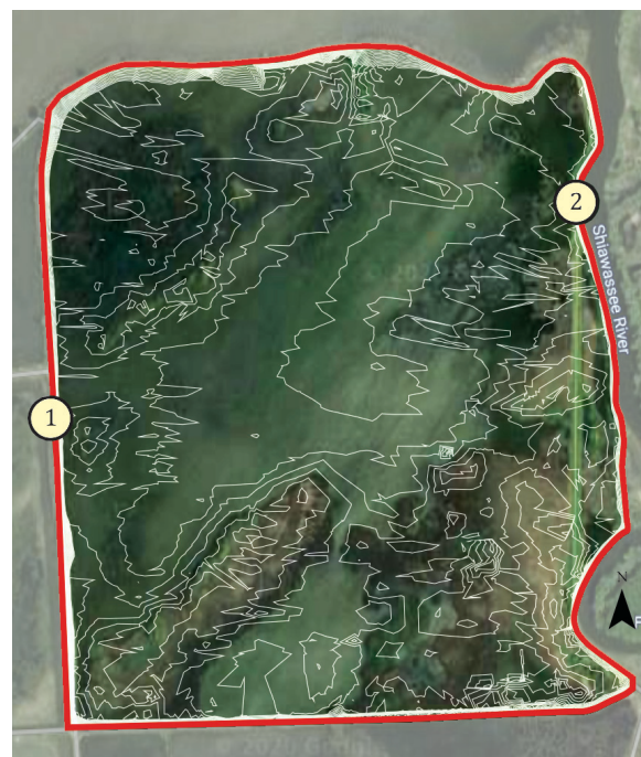
Figure 1.4: Aerial photo of the Pool 1A unit. Gray lines indicate water level topography. Point #1 indicates location of control structure connecting P1A to Maankiki Center; point #2 indicates location of control structure connecting P1A to the Shiawassee River. Image pulled from Lugten et al. (2020).
