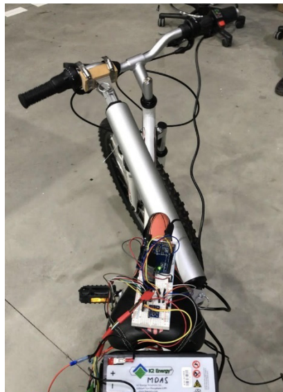
Figure 12: Arduino microcontroller wired to linear actuator.
