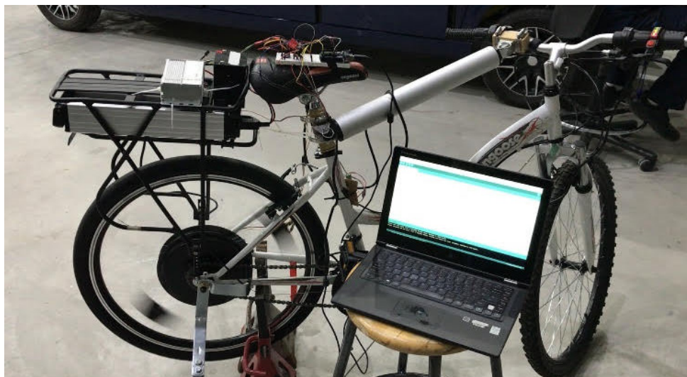
Figure 10: Propulsion system test with the rear wheel raised off the ground.
