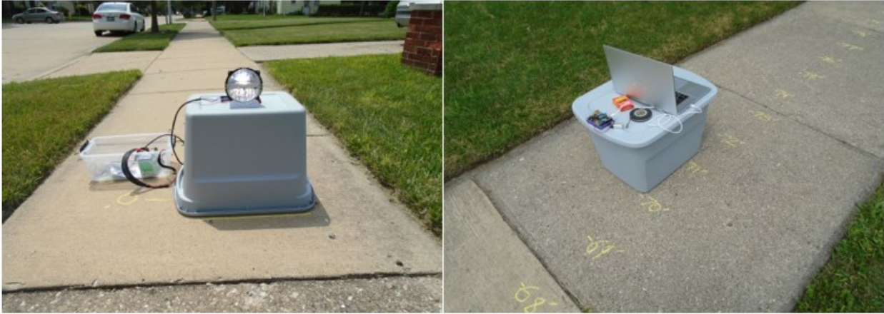
Figure 3.40 Outdoor testing of the VLC prototype in daylight (transmitter, left; receiver, right)
