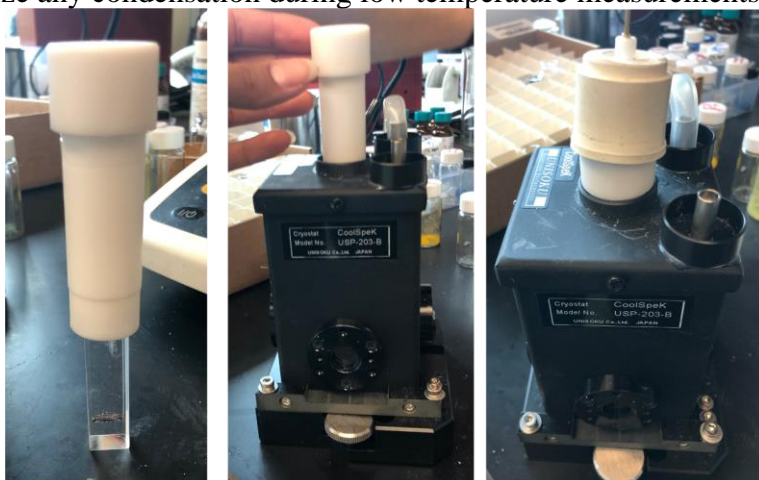
Figure S2. Teflon holder used to grasp 1 cm cuvette and fit snugly inside Cryostat chamber.
