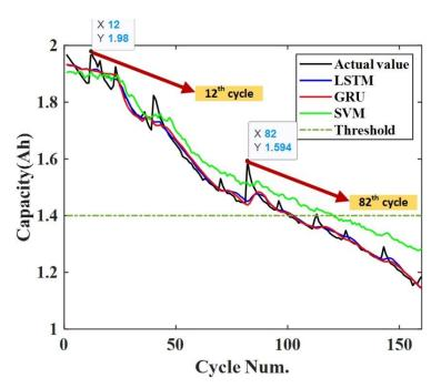
Fig.1: Capacity estimation for Battery #6.
