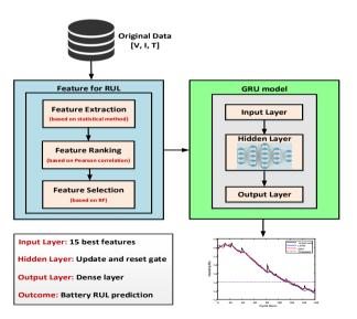
FIGURE 4 Framework of battery remaining useful life prediction.
