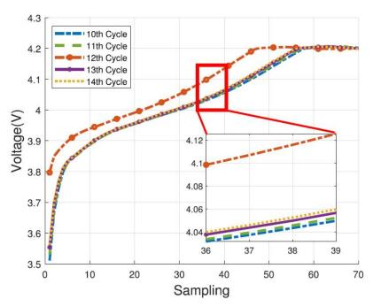
Fig.2: Abnormal voltage pattern at 12th cycle of Battery #6.
