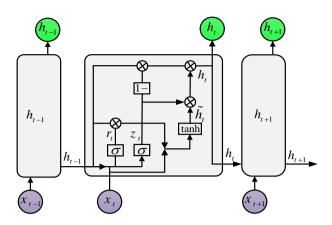
FIGURE 2 The structure of gated recurrent unit memory cell.
