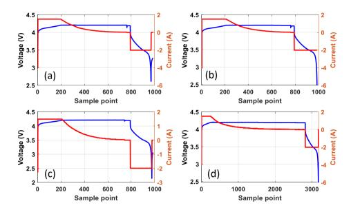
**FIGURE 5** The terminal and current voltage profiles of a charge-discharge life cycle; (a) B0005, (b) B0006, (c) B0007, (d) B0018.
