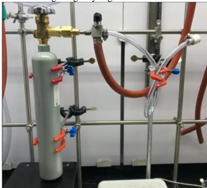
Figure S1. 18 O 2 cylinder Schlenk-line set-up used to minimize air exposure.
