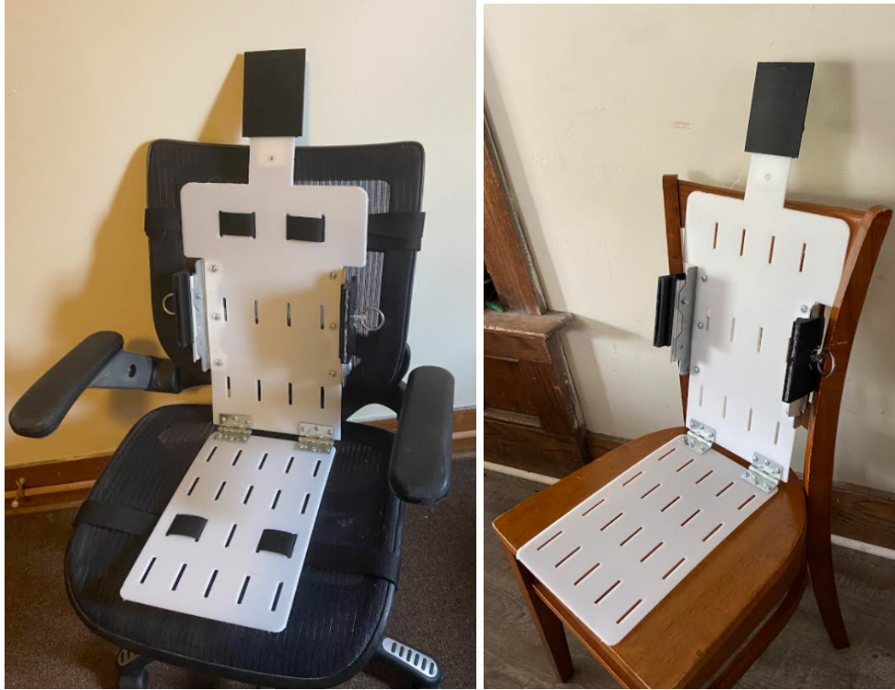
Figure 12: Two views of the full-frame prototype with brackets and adjustable straps.
