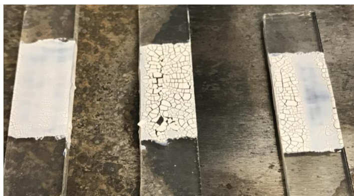
Figure 2. Photoanodes produced prior to reduction in the acetylacetone ratio reduction.
