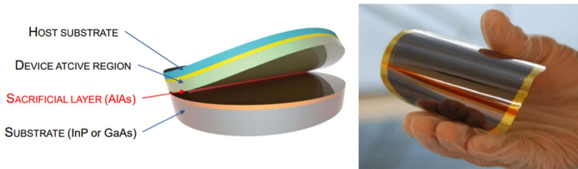
Figure 2: A cross-section of a ND-ELO solar cell shown on the left, and an actual solar cell produced using ND-ELO shown on the right.
