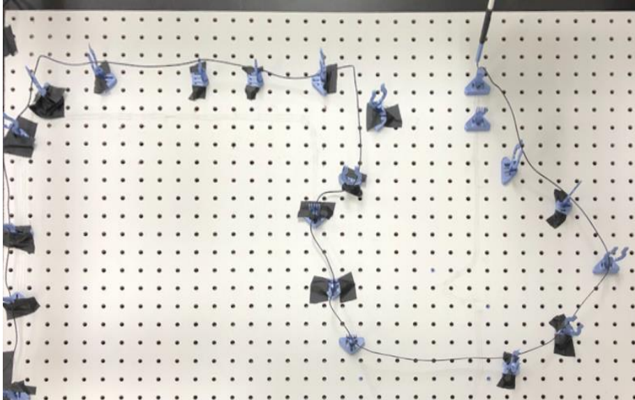
Fig. 9 Overhead view of completed demonstration harness showing various clip designs and clip placements. The extruder tube may be seen in the top right corner.
