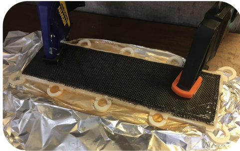
Borosilicate glass clamping 3D-printed molds
