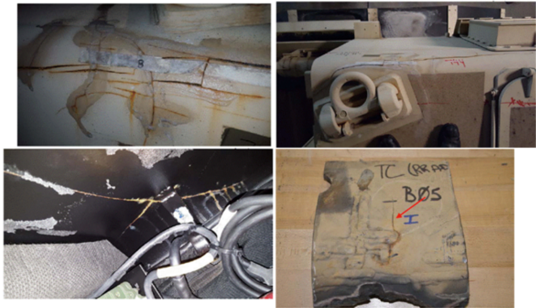
Figure 1.1: Examples of fatigue failure on ground combat vehicles.
