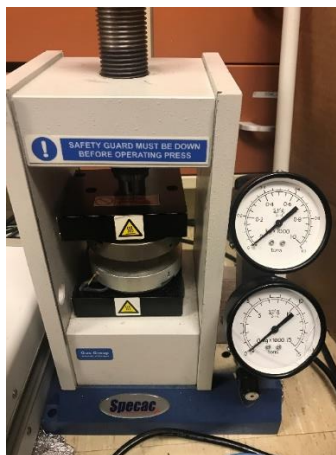
Figure 2-1 A hydraulic manual press tool used for thermal nanoimprint lithography.
