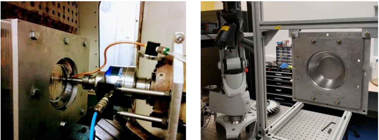
Figure 5.2 (a) Experimental setup for a cone fabrication using TPIF on Cincinnati CNC, and (b) laser scanner set up for part geometry measurement using a Romer Absolute Arm with Integrated Scanner 7525SI
