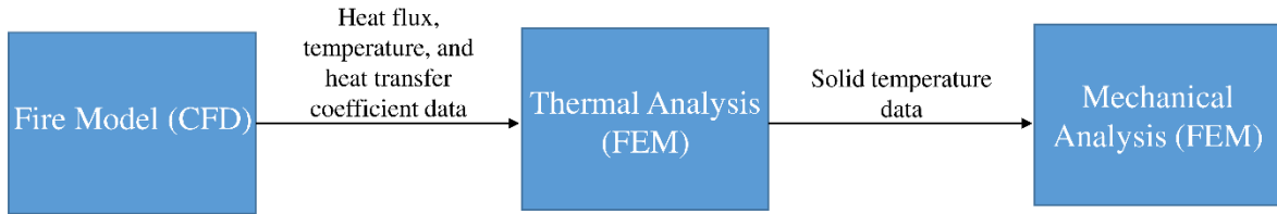
Figure 3.4 - One way (weak) coupling scheme
